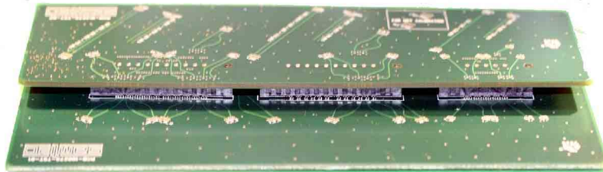
Figure 1 Mated PCB Test Fixture with Mounted Test Connectors
