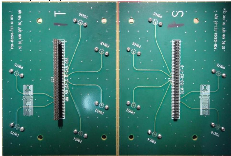
**Series:** MW/CLM**Description:** Surface Mount Board, 1.00mm Pitch, 8.48mm (0.334") stack height
