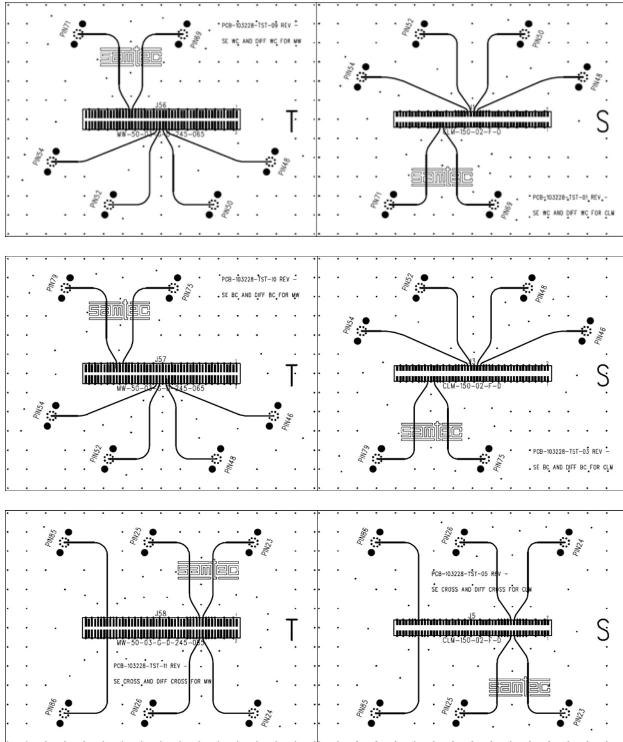
**Series:** MW/CLM**Description:** Surface Mount Board, 1.00mm Pitch, 8.48mm (0.334") stack height
