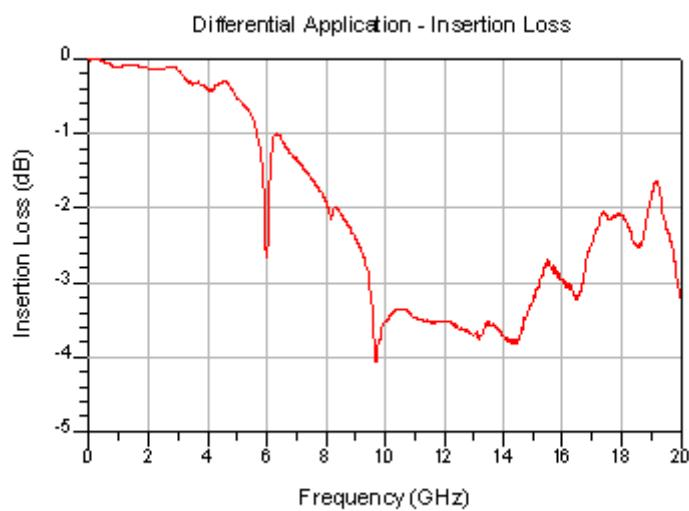
**Series:** MW/CLM**Description:** Surface Mount Board, 1.00mm Pitch, 8.48mm (0.334") stack height
