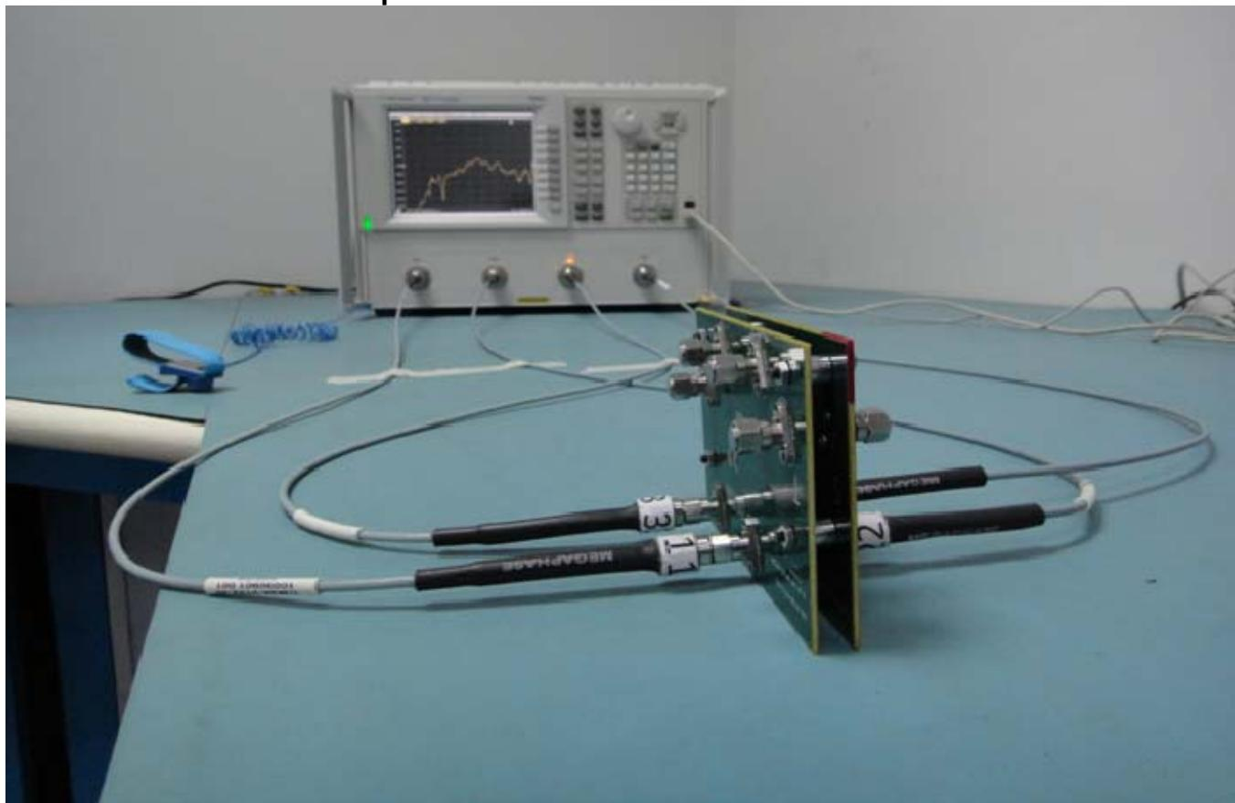
**Series:** MW/CLM**Description:** Surface Mount Board, 1.00mm Pitch, 8.48mm (0.334") stack height**Test Instruments**QTY Description
