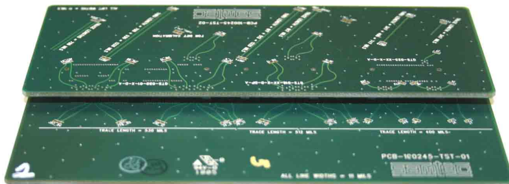
Figure 1 Mated PCB Test Fixture with Mounted Test Connectors
