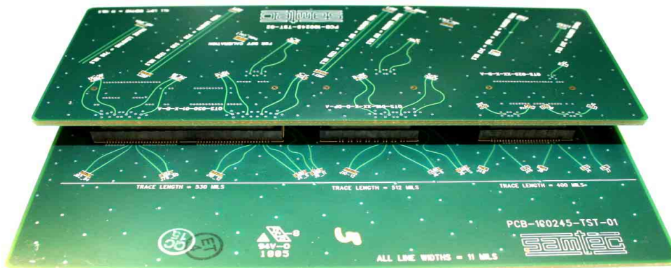
Figure 1 Mated PCB Test Fixture with Mounted Test Connectors
