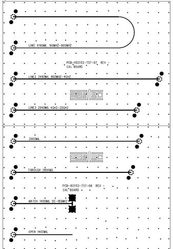
Thru line -2800 mils Open Reflect -1400 mils Line 1 - 6190 mils Line 2 - 3480 mils Line 3 - 2940 mils Match -1400 mils
