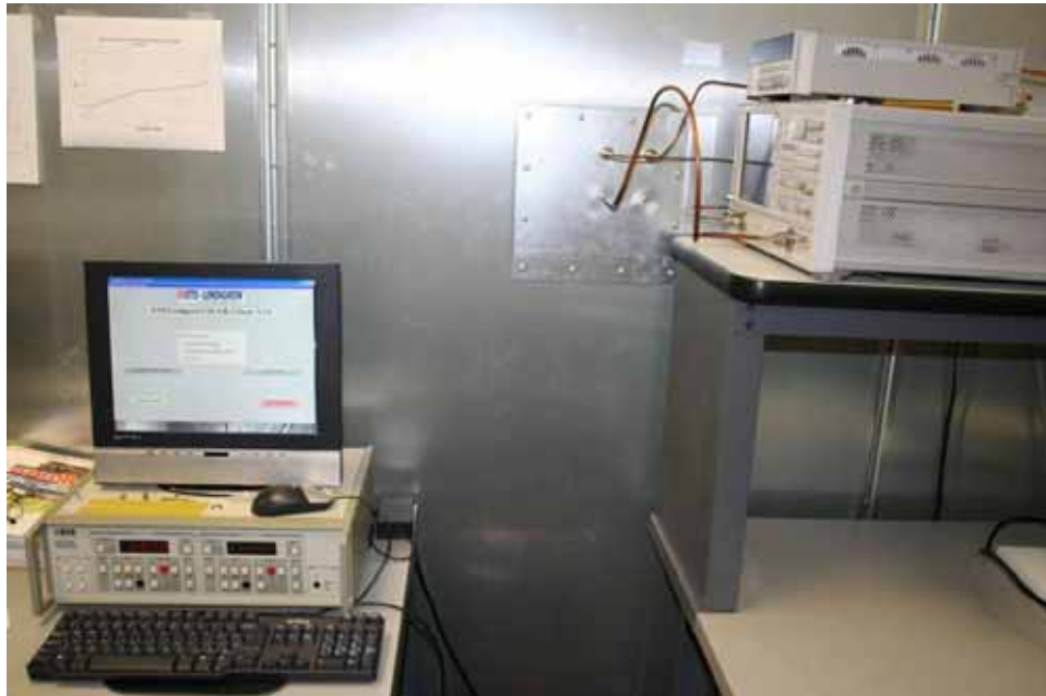
ETS/Lindgren 2090 Multi-Device Controller and HP Vector Network Analyzer
