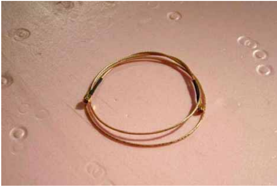
RG-316 single braid coax cable tested for comparison
