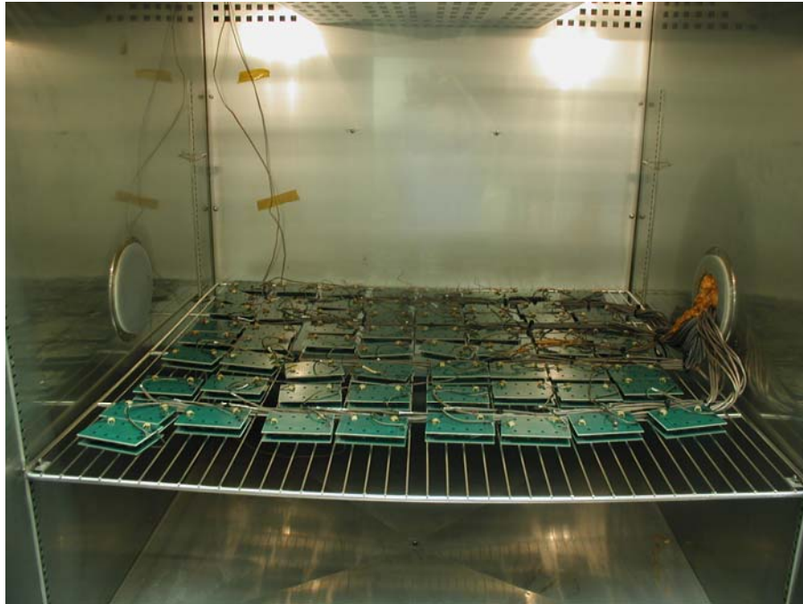
FIGURE 5: Group 1, consisting of 32 mounted mated pair samples of SAC and Group 2, consisting of 32 mounted mated pair samples of SnPb, were monitored. Signal routing was daisy-chained through all 828 positions on each sample facilitating 100% contact monitoring.
