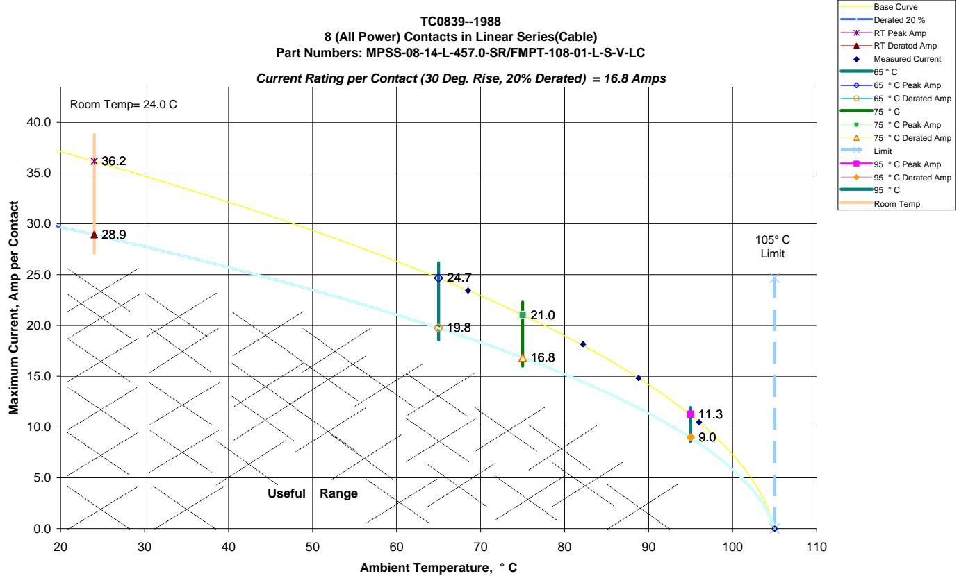
b. Linear configuration with all contacts powered (Thermocouple placed in the contact)
