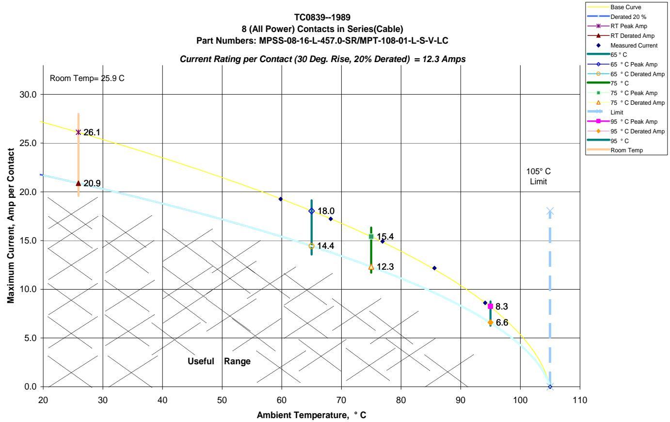
e. Linear configuration with all contacts powered (Thermocouple placed in the contact)
