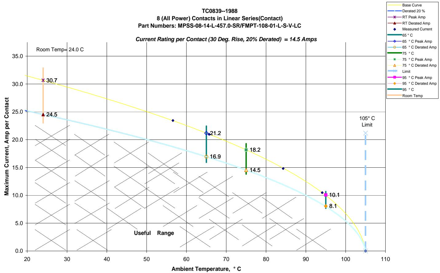
c. Linear configuration with all contacts powered (Thermocouple placed in the crimp)
