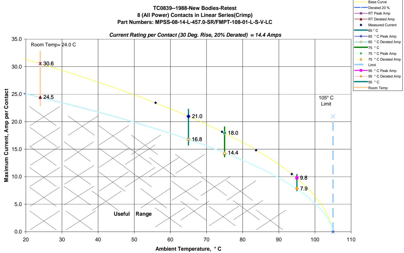
d. Linear configuration with all contacts powered (Thermocouple placed in the cable)
