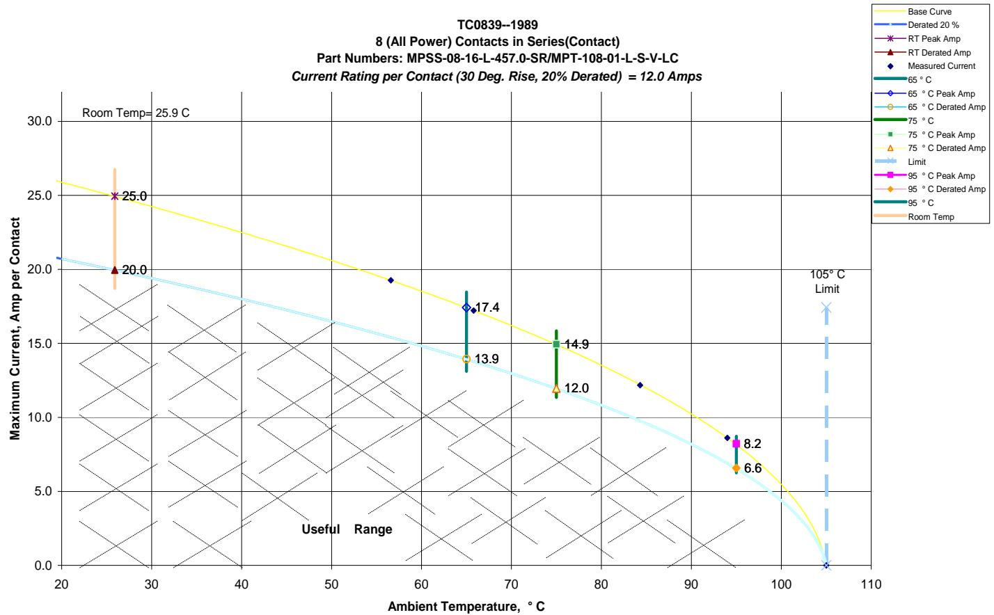
f. Linear configuration with all contacts powered (Thermocouple placed in the crimp)
